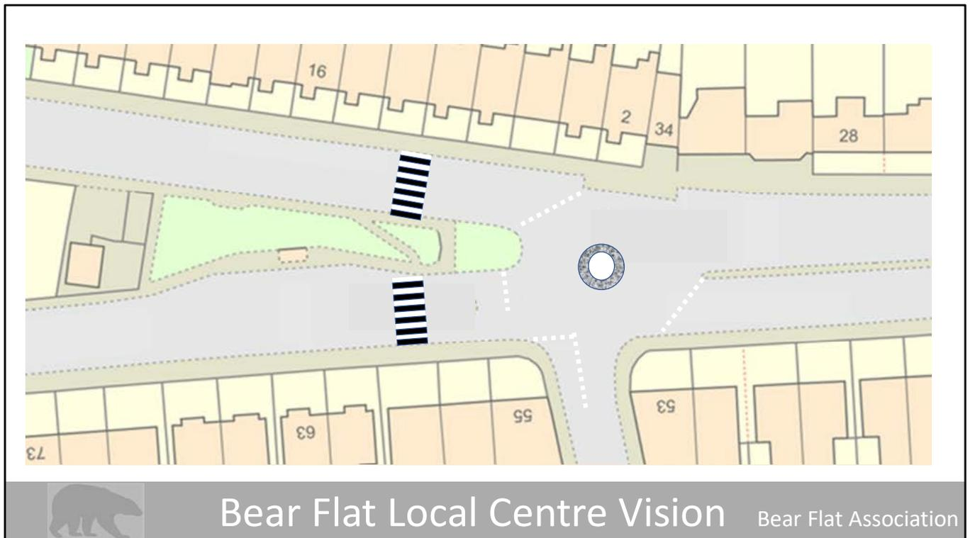
A less expensive approach would be to use a mini-roundabout for traffic control. This should slow traffic and make the junction safer to use.
